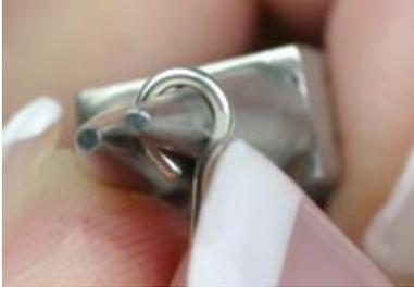
Rotate your wrist away from your body, while using the tip of your thumb on the other hand to push on the wire below the pliers, forming a loop. *The placement of your thumb will help keep the angle sharp and the loop circular.* Turn the wire into a loop.
