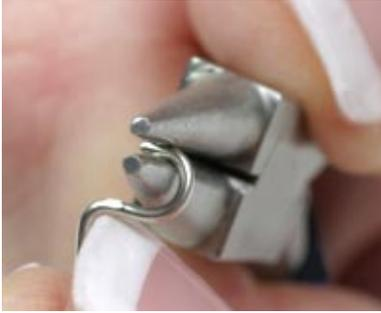
Grip the tip of the wire with the end of the round-nose pliers, leaving very little wire peeking through the barrels of the pliers.
