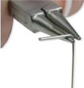
Using round-nose pliers, grip the wire above the last bead added in your design or about 3/8-inch down from the end of a length of wire. Bend the wire to a 90-degree angle.
